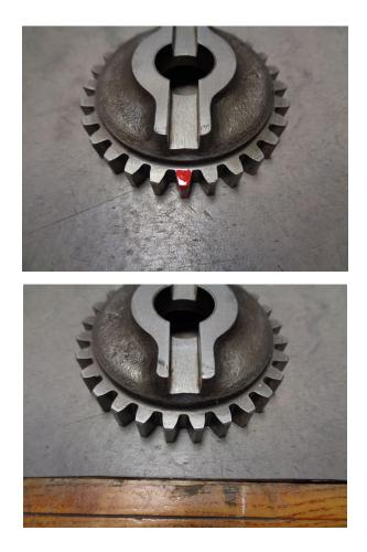
If you install the gear incorrectly you will not be able to time the MAG to the engine, because you will MAX OUT the Ear Slots on the mag BEFORE getting a POINT BREAK.
