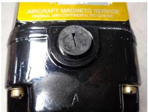
2) The mag direction of rotation is always viewed from the shaft of the magneto. Turn the mag backwards, (clockwise, so that we are not winding up the impulse coupling spring) until you see the RED PAINTED distributor gear tooth enter the timing window. Continue to turn the Shaft until you feel magnetic NEUTRAL (the mag will want to hold this position), and the RED PAINTED tooth will be offset in the window.
