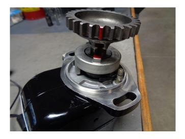
6) With the gear in the correct orientation, install the bushing(must have the machined steel bushing P/N 10-163049, AD74-26-09), split washer, and nut.
